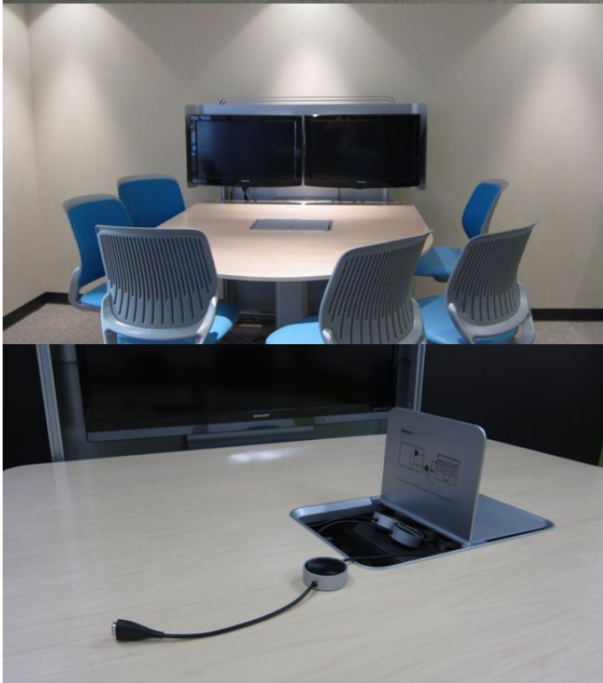
Picture 15: One of the VGA cables for the Steelcase tables. Whether single or dual monitors, the little disk in the VGA cable is what is used to select which laptop is currently displayed. These have proven very easy and extremely popular to use by students.
